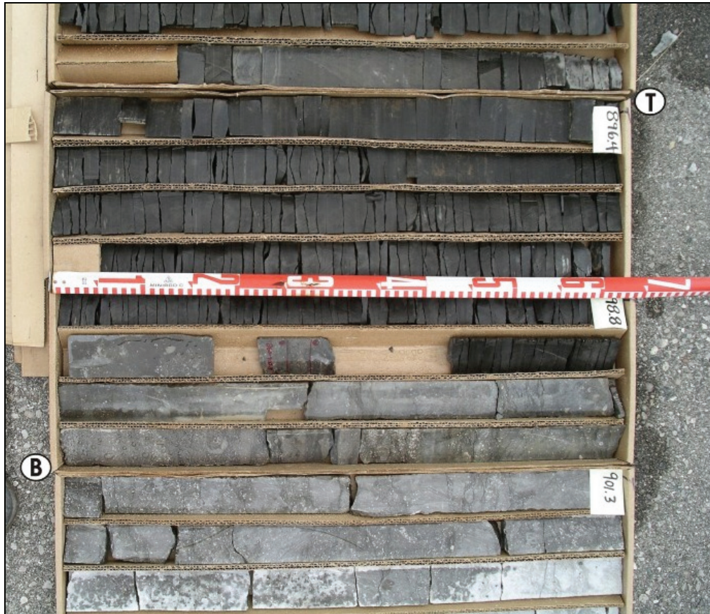
Figure 5.13 Core Disking from Oil/Gas Well in Chatham, Ontario. Section showing is contact between Collingwood and Cobourg formations at from 895 to 908 mbgs (OGS 2006).
